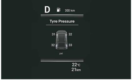
Tyre pressure monitoring system (Highline)
